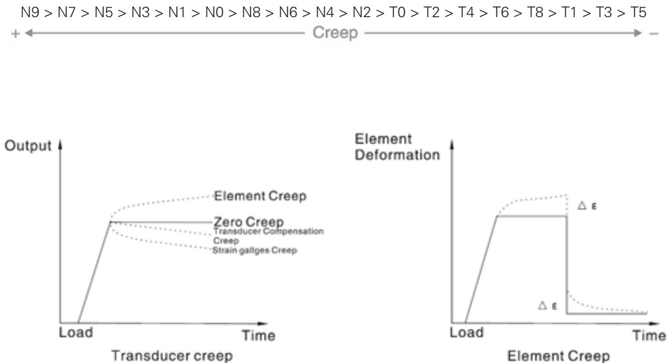
Figure 3: Creep compensation and effect of creep
