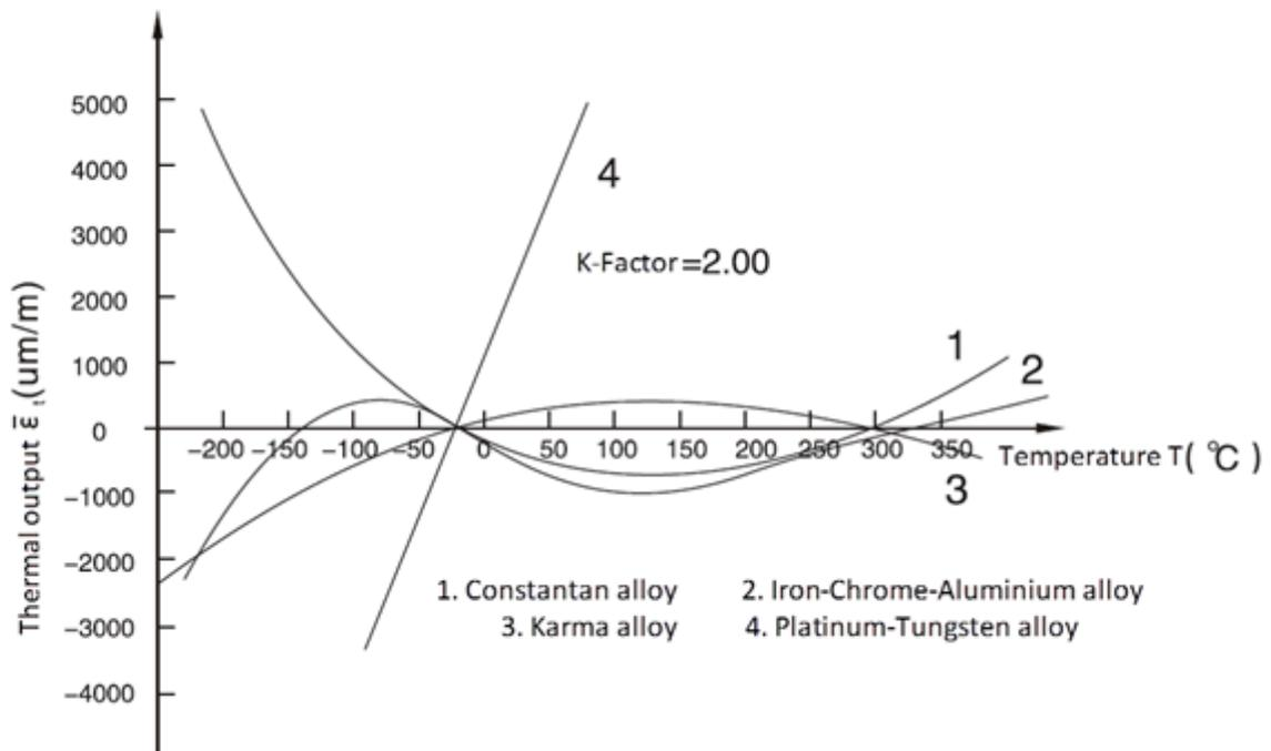
Figure 1: Thermal output curve of strain gauges on different steel materials
