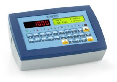
High performance digital weight indicator, with 3 serial ports, transmission protocols for data communication, completely configurable printouts, integrated alibi memory, graphic display and port for connection to barcode/badge reader. The wide range of connectable accessories and printers guarantees the maximum interfaceability and versatility. CE-M approvable (OIML R-76 / EN 45501).
