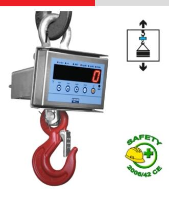
Stainless steel crane scales, with large 40mm DOT LED display, for maximum visibility from any angle and in any light condition, also with direct sunlight. The single security system makes them suitable for lifting and weighing the load. Sturdy and reliable, usable in any environment, inside or outside. Minimum reduction of the lifting space of the crane. IP67 protection, from dust and rain. Available also CE-M APPROVED. Fitted with test certificate obtained with sample weights.
